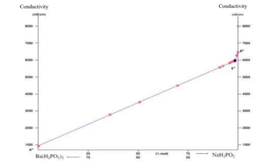
Figure 3. Yeneke – Le Chatelier diagram of the conductivity of NaH<sub>2</sub>PO<sub>2</sub>-Ba(H<sub>2</sub>PO<sub>2</sub>)<sub>2</sub>-H<sub>2</sub>O ternary system.
