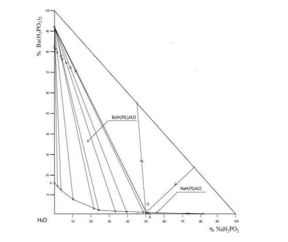
Figure 1. Solubility and phase equilibria diagram of  $NaH_2PO_2$ -Ba $(H_2PO_2)_2$ -H<sub>2</sub>O ternary water-salt system at room temperature (the Rozeboum method).
